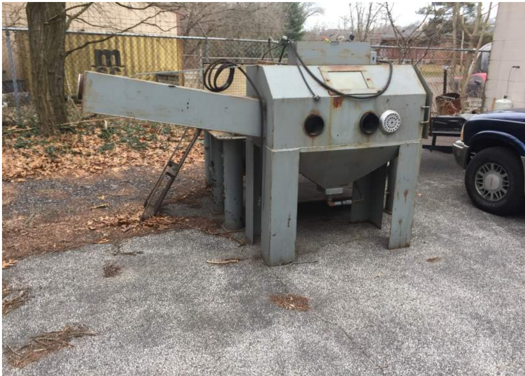
Photo 17: Sandblasting equipment on south portion of Subject Property
